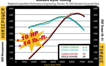
Max. Gain = 10 hp & 14 lb-ft from 3630 to 3690 rpm Peak Gain = 4 hp & 8 lb-ft at 6100 rpm
